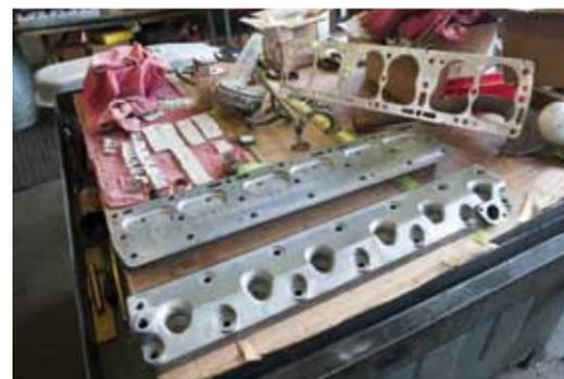
In this Ohio shop, things mostly happen in pieces, not necessarily as an integrated whole. Main bearing caps and bolts for Packard V-12s are cast and machined. Axles, brake and hub assemblies are renewed. So are Packard V-12 cylinder heads during a buildup.
