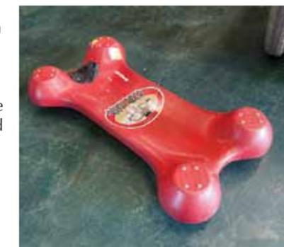
This is a comfortable way to do shop work. The Bone floor creeper, made of molded plastic, is a main enterprise for Dale.
