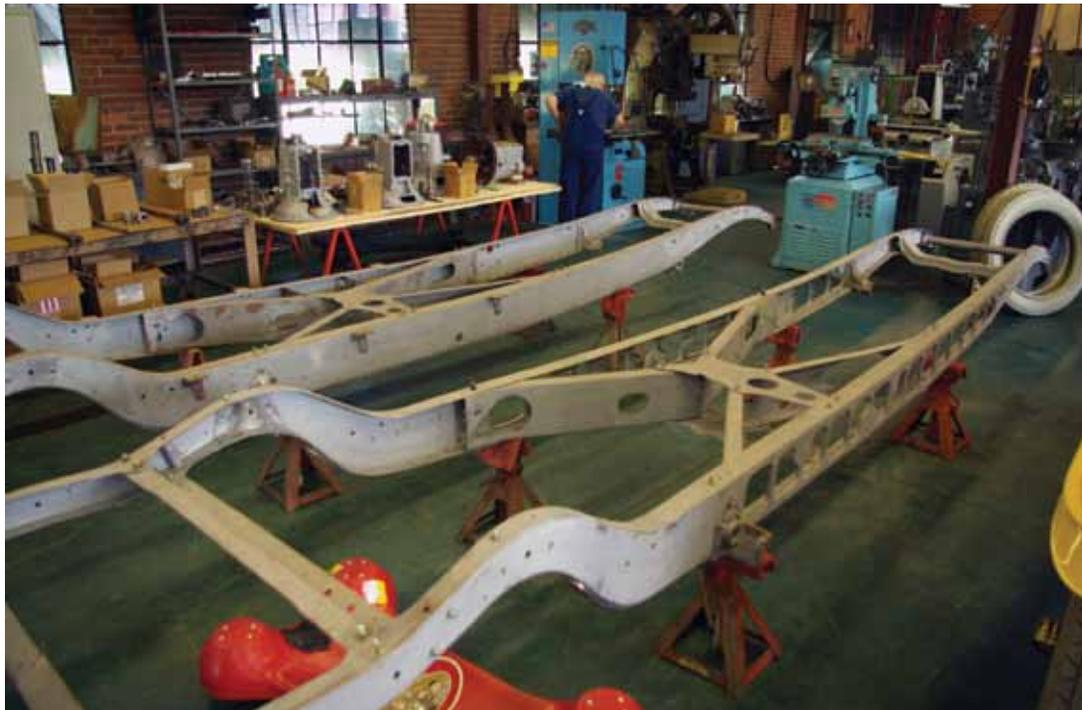
**Custom bodies require special components underneath. One such project cooking in Dale's mind would combine a pair of 1934 Graham superchargers with a stoutly modified version of the shop's specialty, a rebuilt Packard V-12. The frame in the foreground, with lightening holes that would do any early dragster or dry lakes car proud, is another element.**
